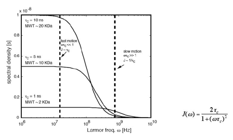
Fig.: the spectral density or the efficiency of relaxation for different Larmor frequencies and rotational correlation times  $\tau_c$ .
