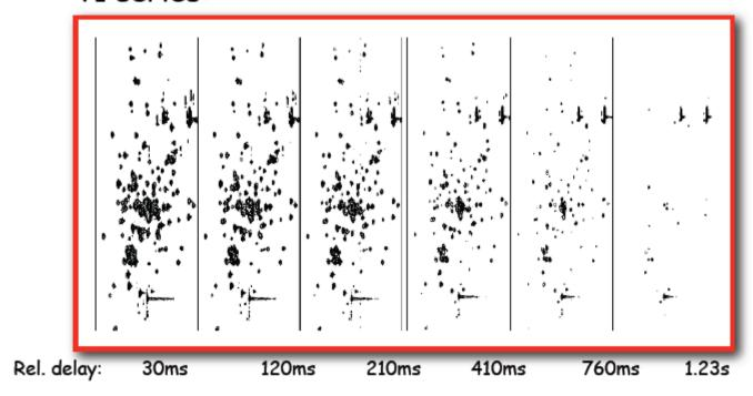
Record a series of  $^{1}\text{H}$ ,  $^{15}\text{N}$  2D spectra, in which the intensity of the peaks is modulated by relaxation
