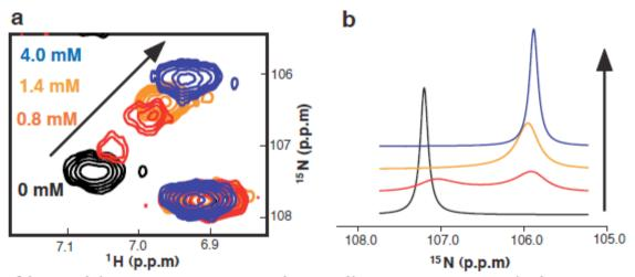
Titration of ligand (concentration indicated) into protein. A) shows a peak from the protein HSQC undergoing the transition from free to bound. B) shows the 1D lineshape simulation of the spectrum.
