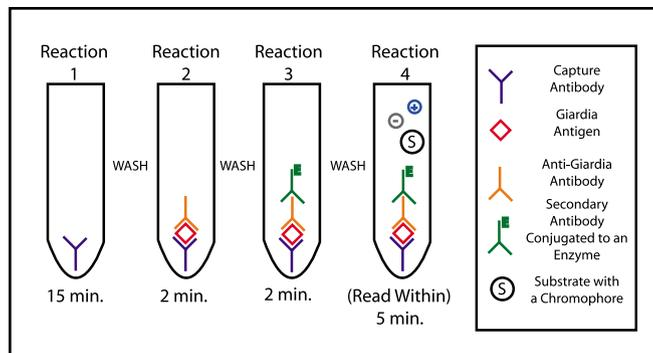
**Figure 3** A schematic of the GiardEIA capture (sandwich) assay used to detect *Giardia lamblia* antigens in fecal samples. The test takes less than 30 minutes to complete.
