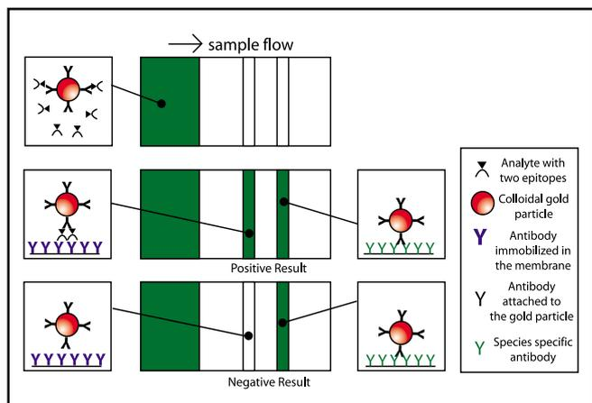
**Figure 5** A schematic of a lateral flow capture (sandwich) assay used for detection of analytes (like hormones) with multiple epitopes.
