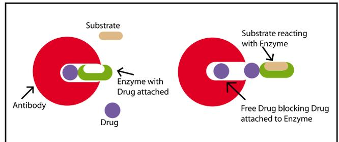
**Figure 7** Enzyme multiplied immunoassay (EMIT) for the measurement of free drug in the sample involving a fixed quantity of enzyme-bound drug, and an anti-drug antibody. After substrate addition, the development of color is measured at 15 and 45 seconds, and the change in absorbance is converted into a concentration reading using a standard curve based on known amounts of free drug in solution.
